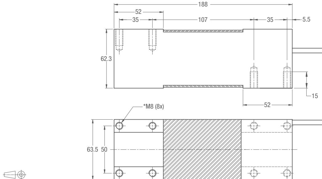
Mounting bolts M8 8.8; torque 25 Nm. Torque value assumes oiled threads.
